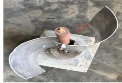
Fig. 2: Fabricated Two-bladed Savonius Rotor.
