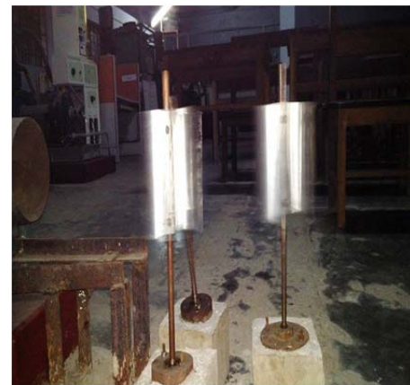
Fig. 4: Cluster of three 2-bladed Savonius wind rotors.(Front View)
