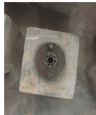
Fig. 1: Cubic block with base at top
