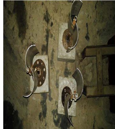
Fig. 3: Cluster of three 2-bladed Savonius wind rotors.(3-D view)
